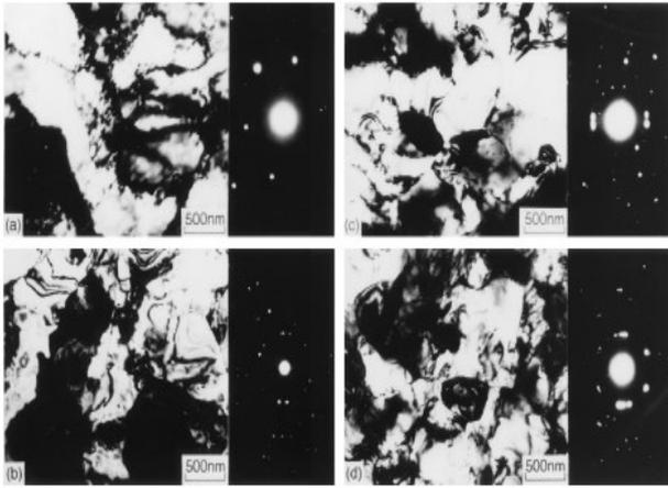
**Figure 15 TEM images and diffraction pattern of the alloy specimens after a) one cycle, 50% reduction, b) 3 cycles, 87.5% reduction, c) 6 cycles, 98.4% reduction, and d) 7 cycles, 99.2% reduction [13]**
