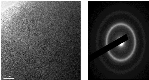
**Fig 20 Microstructure of the alloy in amorphous state.**
