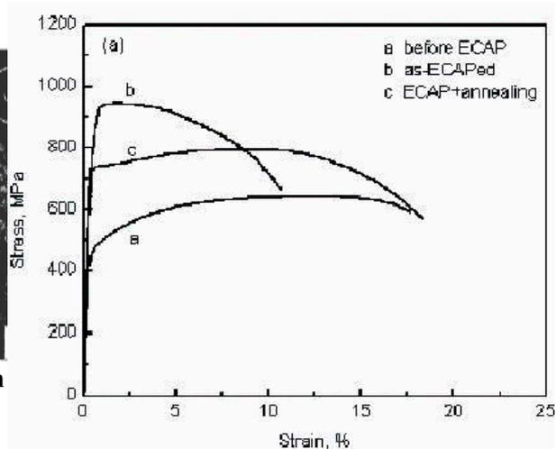
Figure 7 Stress- strain curves of vanadium alloyed steel [8]
