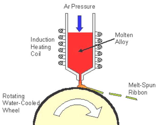
**Figure 16** Melt- spinning process [16]
