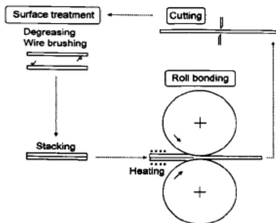
Figure 13 Accumulated roll bonding (ARB) method [13]
