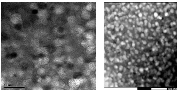
**Fig 21 Microstructure of the alloy in crystalline state, a) TEM and b) STEM image.**
