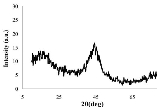
Fig 18 XRD pattern of  $\text{Fe}_{55}\text{Cr}_{18}\text{Mo}_7\text{B}_{16}\text{C}_4$  in amorphous state.
