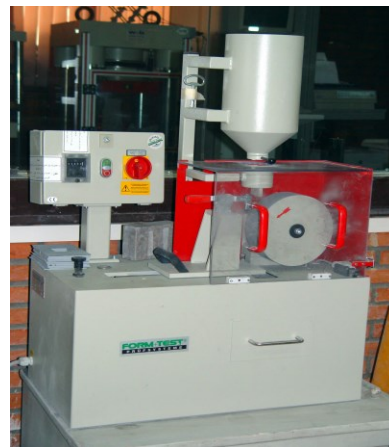
Fig 3 Abrasion test apparatus based on EN standard
