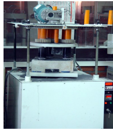
Fig 2 Manufactured revolving disk apparatus based on ASTM standard
